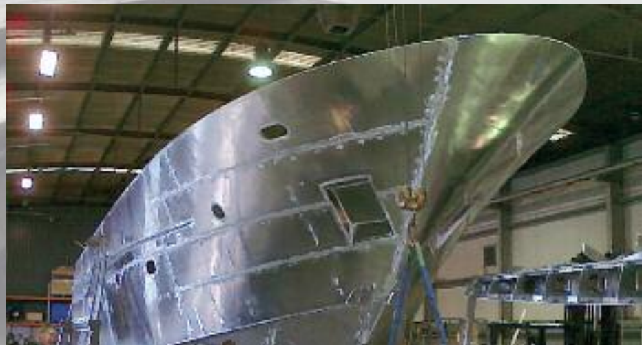
Work on an aluminium hull
